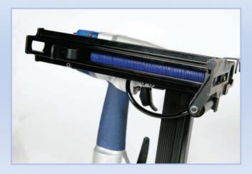
The pneumatically powered Tagaplus Cap Stapler uses plastic staples to affix a plastic reinforcing cap or disk over timber wrap to prevent the cover from tearing through the staple. The 10mm staples and the 25mm diameter caps are automatically fed from the tool magazines during the tool cycle.
